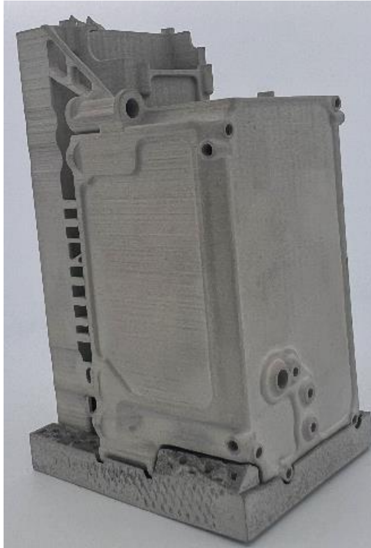
Figure 1 Fluid Matter Exchanger sintered on a sintering live-setter.
