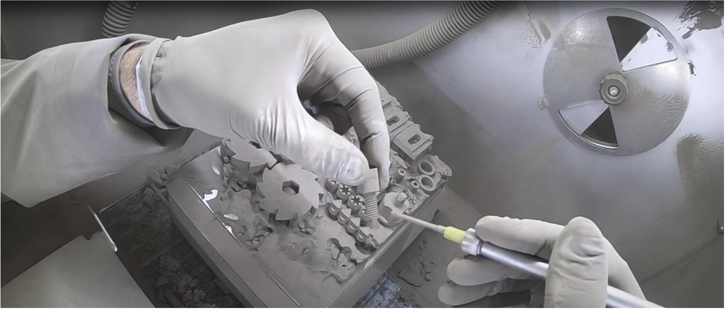
Figure 7 “Depowdering” process of Metal Binder Jetting (a.k.a. “Decaking”). Process consists of removing excess powder manually with the assistance of compressed air.
