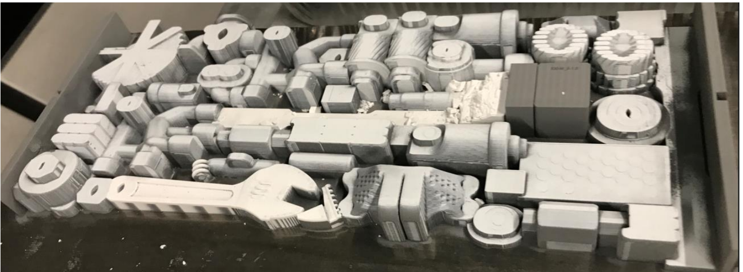
Figure 8 “Support Removal” process of Metal Material Jetting (a.k.a. “Decaking”). Process consists of dissolving the support material by immersion of the entire build in citric acidic solution, and then manually rinsing the parts in water.
