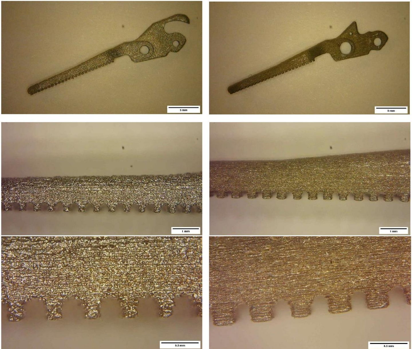
Figure 9 Typical feature resolution comparison between Metal Binder Jetting (left) and Metal Material Jetting (right).
