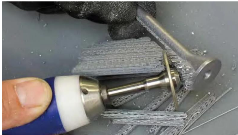
Figure 7 Laser powder bed fusion: supported much be machine away (Image credit: Conteo AG)
