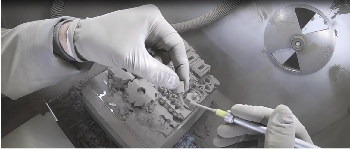
Figure 6 Metal binder jetting: Parts are printed floating in powder, no support required. (Image: Azoth)
